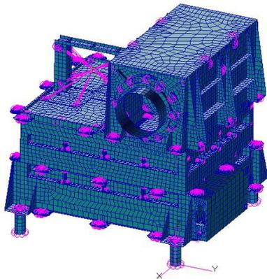
Figure 1: Finite element model of the EPT-HET instrument
