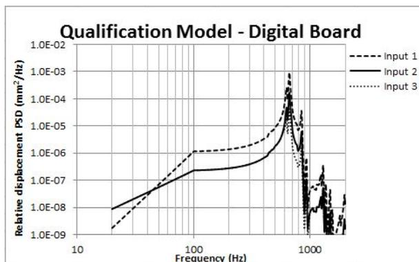
Figure 2: Relative Displacement Spectral Density (RDS) curves for three different random excitations
