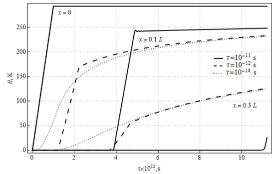
Figure 1: Time variations of temperature increment  $\theta$  at positions  $x = 0, x = 0.1L$  and  $x = 0.3L$  for the PZT-4 bar for values of relaxation time  $\tau = 10^{-11}, 10^{-12}, 10^{-14} s$ .
