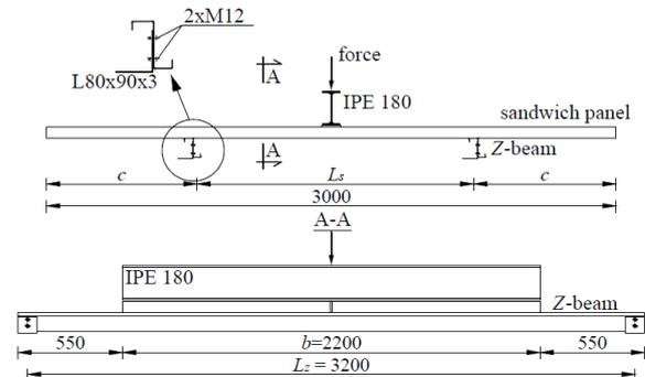
Figure 1: Scheme of the test-bed
