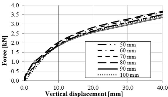
Figure 3: The comparison of vertical displacement of thin-walled element in dependence of the thickness of the sandwich panel.
