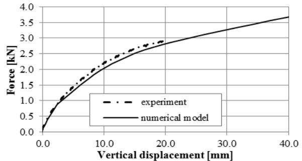
Figure 2: The dependence of the force and vertical displacement in the middle of the thin-walled element
