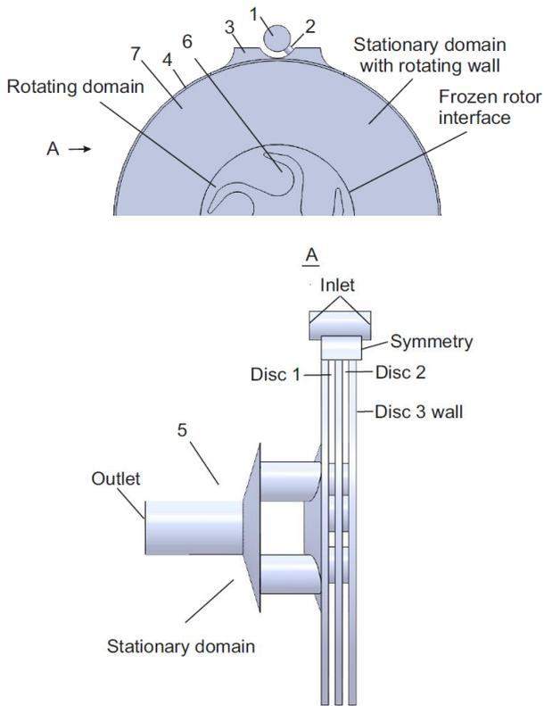
Figure 1. Calculation domain and most important boundary conditions
