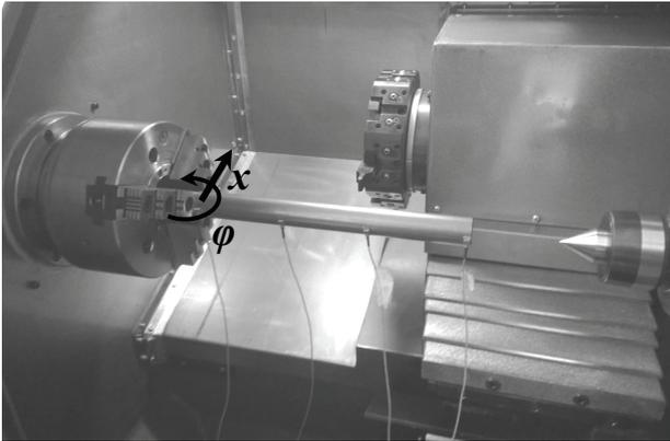
Figure 1: Lathe spindle holder with testing rod
