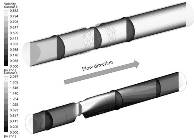
Figure 4: Velocity profile comparison for two analysed cases
