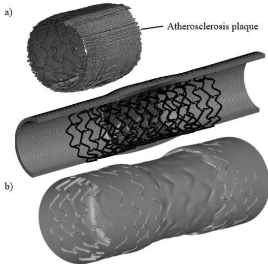
Figure 2: Models used to create the domains: a) FEM from the last step of the implicit analysis, b) Geometry of the domain after implanting the stent
