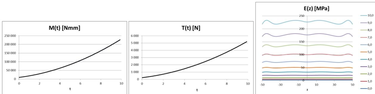
Figure 2. The Young modulus  $z$ -distribution in time using permanent loading program
