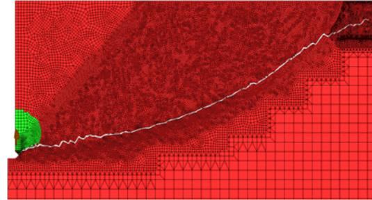
Figure 5: Crack path obtained using element deletion method
