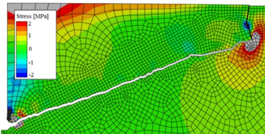
Figure 4: Maximal principal stress distribution and crack propagation path in FEA model for 20 cm anchor using X-FEM method. Stress greater than  $f_t = 2$  MPa is omitted.
