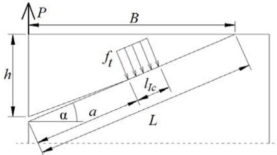
Figure 3: Scheme for calculation of the critical force  $P$
