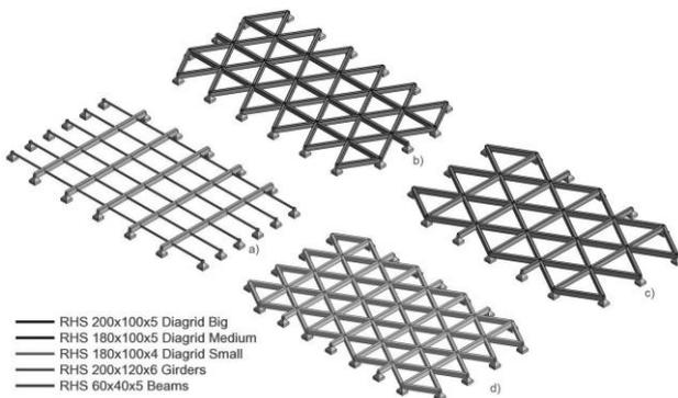
Figure 1: Examples of the grillage structure: a) orthogonal, b) diagrid medium, c) diagrid big, d) diagrid small
