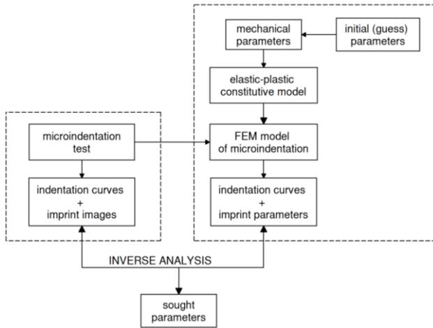
Figure 1: The inverse problem framework of the calcium deposit mechanical characterization
