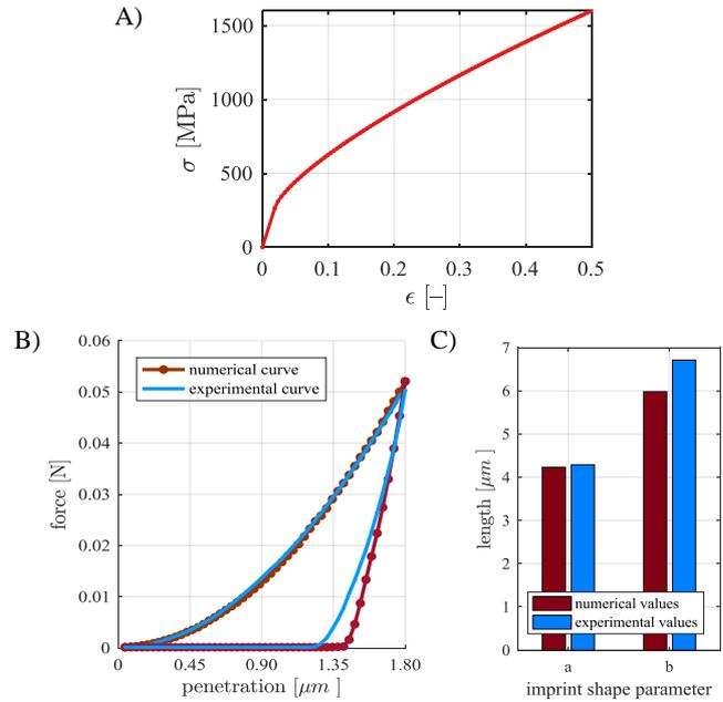
Figure 2: Constitutive law identified in the study (A), comparison between experimental and numerical counterparts: indentation curves (B) and imprint shape parameters (C)
