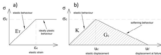
Figure 2: Material models - a) timber (simplified), b) cohesive
