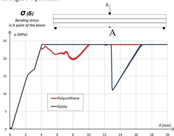
Figure 4: Bending stress - vertical displacement relation
