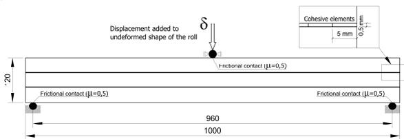
Figure 1: Three layer glue laminated timber beam model
