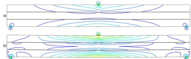
Figure 6: Huber - Mises stress isolines plot, a) before delamination, b) during delamination
