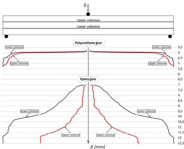
Figure 5: Cohesive crack propagation - displacement relation
