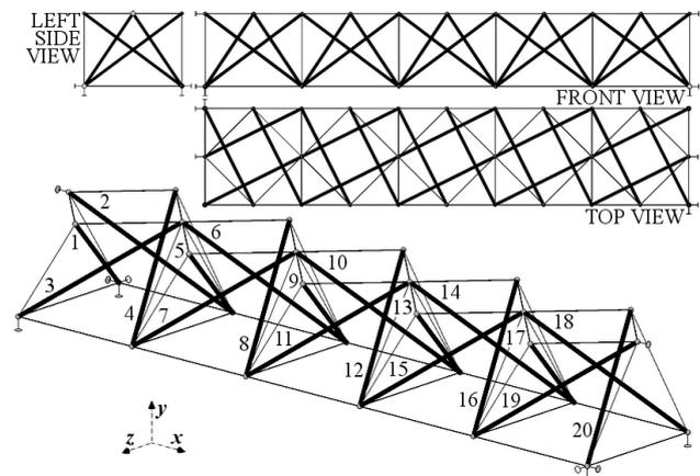
Figure 1: Plot of analysed tensegrity girder with numbered active members (thick members)
