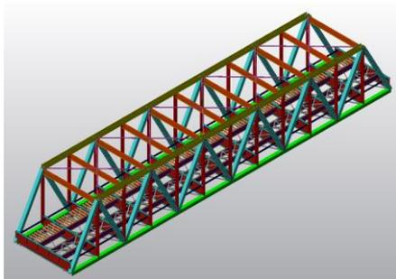
Figure 4: A three-dimensional spatial model of the railway bridge.
