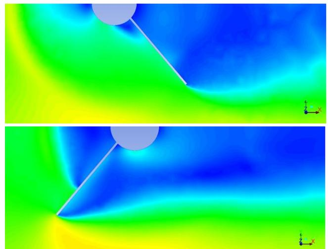
Figure 4: Wind flow patterns at height 15 m: top – diverging, bottom – converging case
