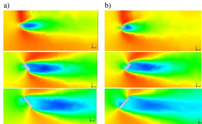
Figure 3: Wind flow patterns at height: 37 m, 33 m and 25 m: a) diverging, b) converging case
