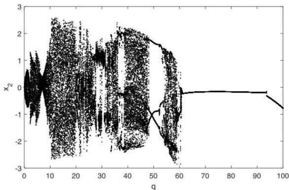
Figure 2: Bifurcation diagram of  $x_2$  vibrations
