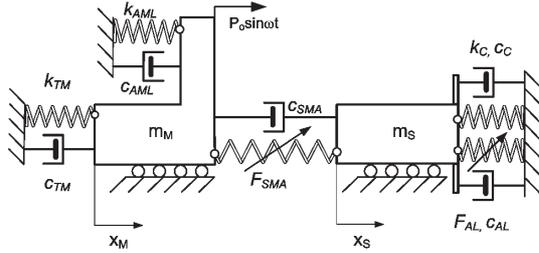
Figure 1: Two degree of freedom model with SMA element
