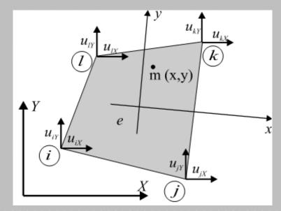
The nodes of this element are locally numbered: i, j, k, l and they have their global numbers resectively: n<sub>i</sub>, n<sub>i</sub>, n<sub>k</sub>, n<sub>l</sub>.
