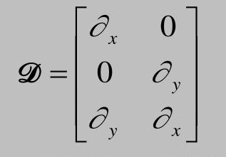
$\mathcal{D} = \begin{bmatrix} \partial_x & 0 \\ 0 & \partial_y \\ \partial_y & \partial_x \end{bmatrix} \quad \text{with respect to } x: \quad \partial_x = \frac{\partial}{\partial x}$ and  $\partial_y$  with respect to y. where  $\partial_{x}$  signifies differentiation
