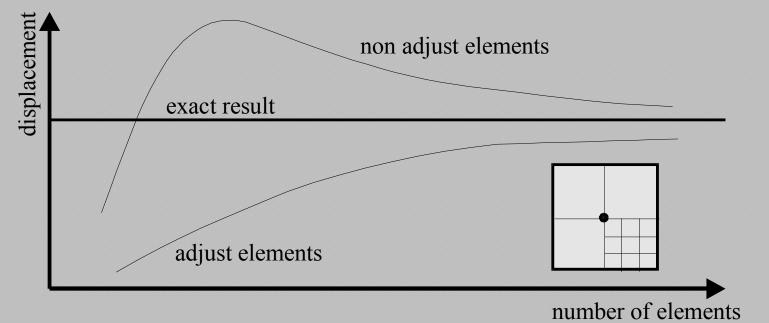
The precision of calculations for incompatible and nonincompatible elements depending on the number of elements.
