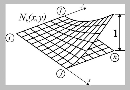
The deformation of the element surface whose the k node is displaced by a unit in the direction perpendicular to this element.
