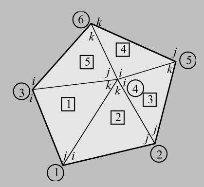
This is a plate divided into five triangular elements. The plate has six nodes numbered from 1 to 6, every element has a local notation of nodes i, j, k.
