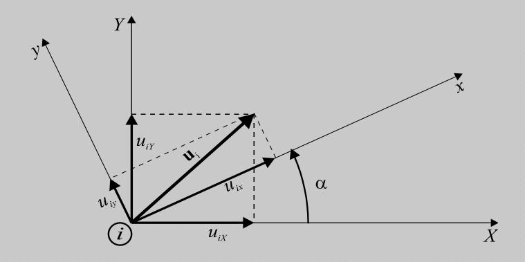
Displacement vector components in the global and local coordinate systems rotated through the  $\alpha$  angle
